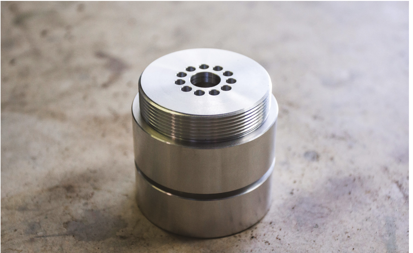
A CNC steel part made using a lathe
