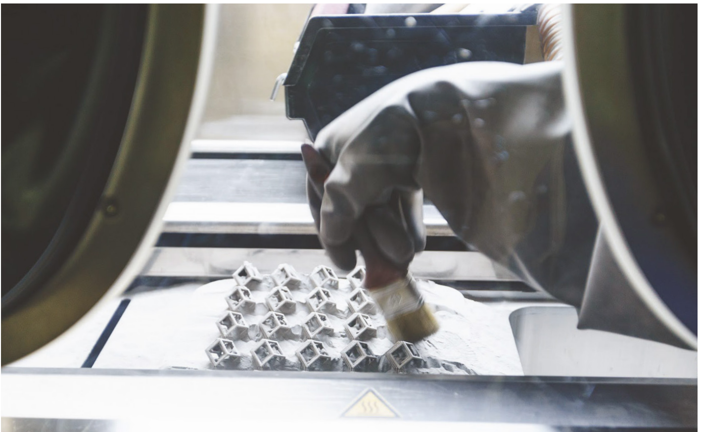
Powder removal after printing. Build plate contains 20 custom parts in steel.
