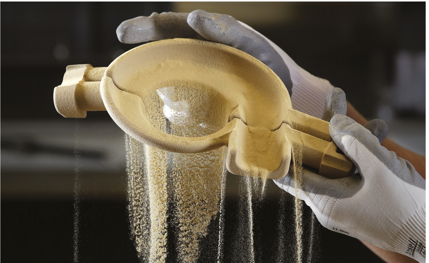
Binder jetted part taken out of the powder. Image courtesy of ExOne.
